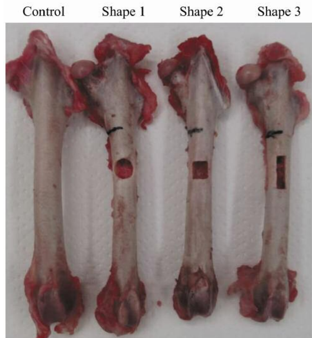
Figure 2. Representative specimens demonstrating the artificially created bone biopsy hole in groups. Control: No defect. Shape 1: Round hole. Shape 2: Square hole. Shape 3: Rectangular hole.
