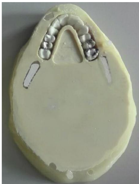
Figure 3. Slice of the upper jaw with metal implants (one molar and two premolars) corresponding to layer 8.
