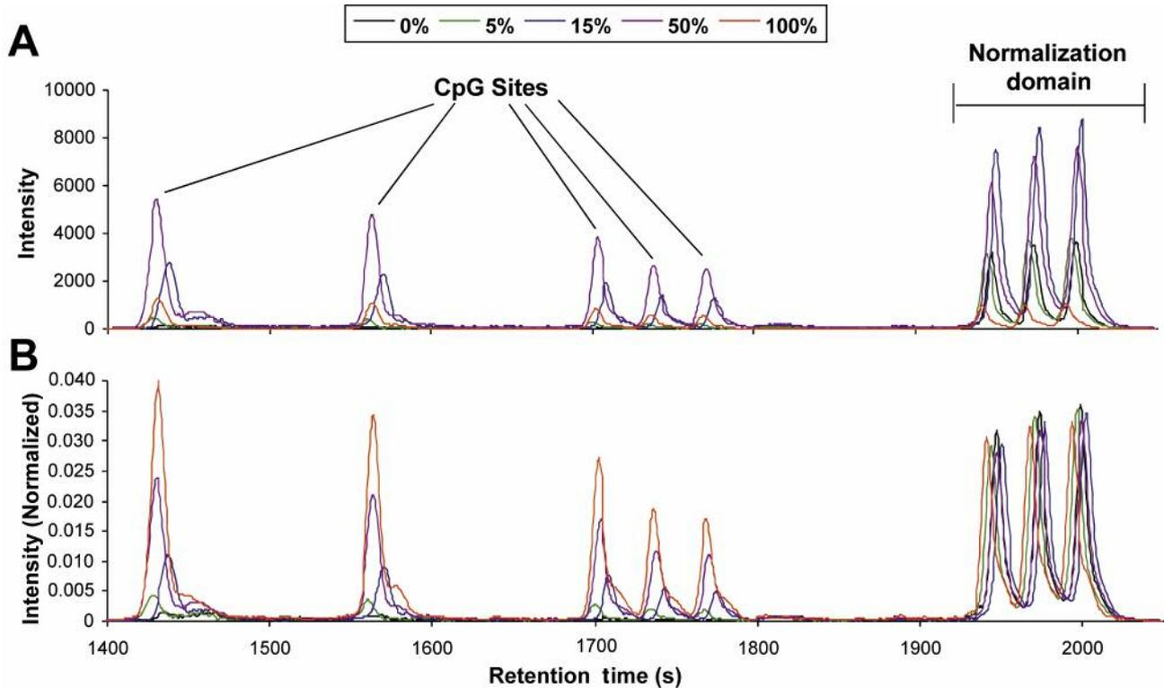
Figure 1. Principle of signal normalization. Sequence electropherograms (cytosine traces only) from five mixtures of methylated and unmethylated DNA (0, 5, 15, 50, and 100% methylated DNA) before (A) and after (B) signal normalization. Normalization is achieved by dividing the intensity by the area of the normalization signal.
