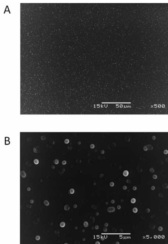
Figure 2. Surface of soft-polymer sheet for photosensitization. Close-up of the surface of the polymer (A) and higher magnification (B). The polymer sheet contained photosensitizer and the protruding brushes.
