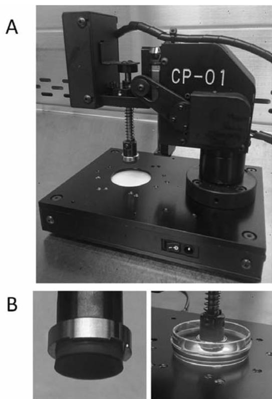
Figure 1. Printing system with a photosensitizer and brush-shaped soft-polymer sheet. The whole system (A) and soft-polymer sheet (B) are shown. A sterilized sheet was applied directly on top of the culture dish by the cylinder and activated by illumination of a light-emitting diode (C).
