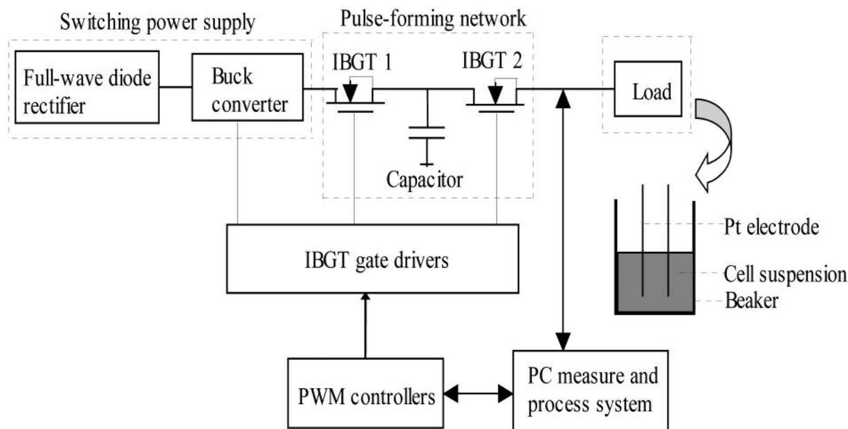
Figure 1. Schematic diagram of steep pulsed electric field generator. The diameter of the beaker was 3 cm; height was 5 cm. Distance between the two electrodes was 1 cm.
