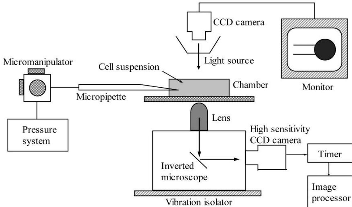
Figure 3. Schematic diagram of micropipette aspiration system.
