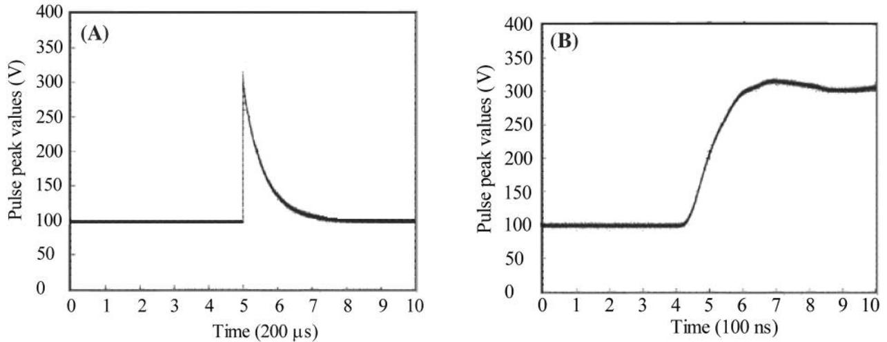
Figure 2. Full waveform (A) and rising edge (B) of steep pulsed electric field (SPEF) produced by the generator.
