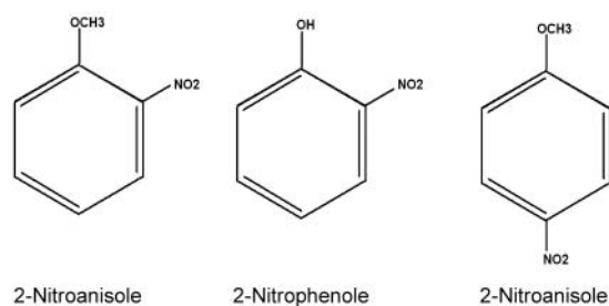
Figure 8. Structural formulae of 2-Nitroanisole, 2-Nitrophenol and 4-Nitroanisole.
