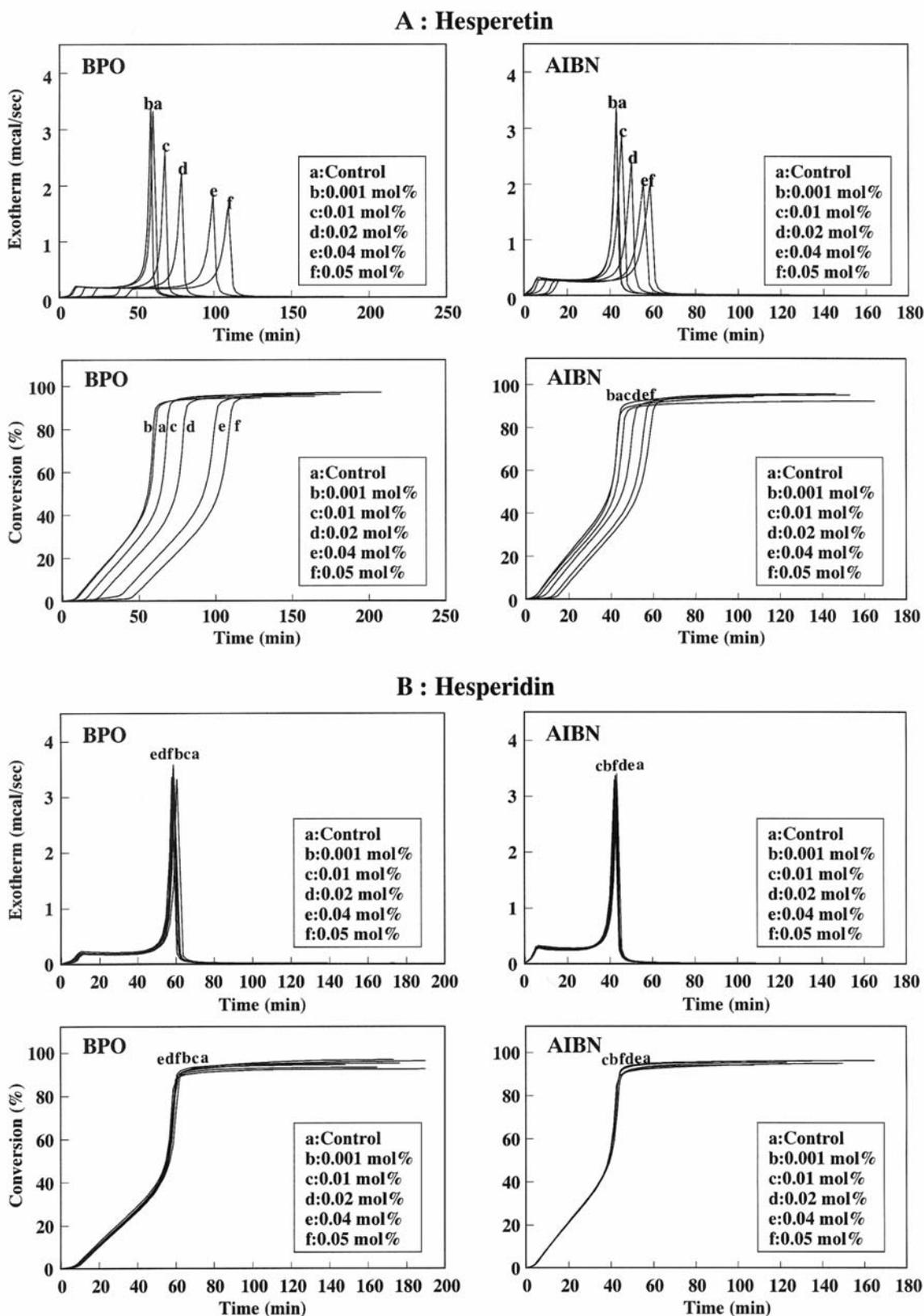
Figure 2. Exothermic (top) and time-conversion (bottom) curves for the polymerization of methyl methacrylate initiated by the thermal decomposition of AIBN and BPO in the presence of hesperetin (A) and hesperidin (B).
