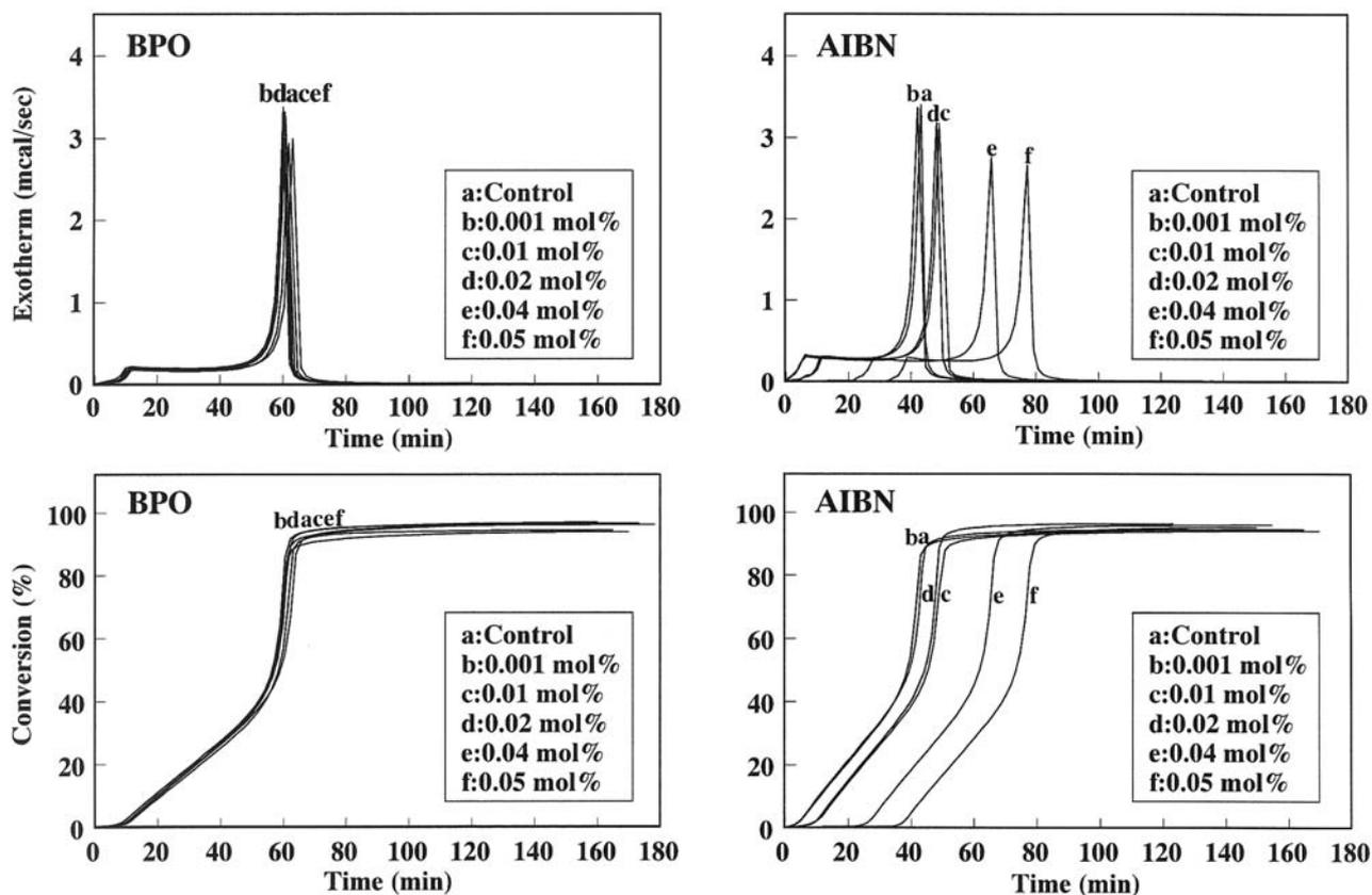
Figure 3. Exothermic (top) and time-conversion (bottom) curves for the polymerization of methyl methacrylate initiated by the thermal decomposition of AIBN and BPO in the presence of trolox.
