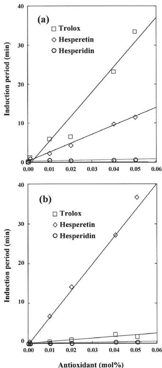
Figure 4. Plots of induction period vs. concentrations of hesperetin, hesperidin and trolox in the polymerization of methyl methacrylate initiated by thermal decomposition of AIBN (a) and BPO (b).
