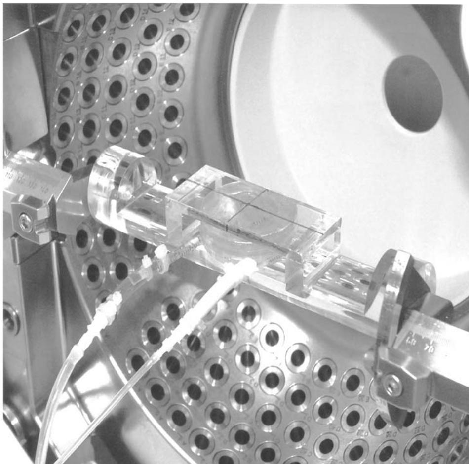
Figure 1. Leksell Gamma Knife® model "B" (Elekta Instruments, Atlanta, GA USA) with attached "cell irradiator" device.
