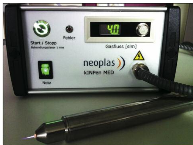
Figure 1. The atmospheric pressure argon plasma jet kINPen MED. The jet excites a flux of argon gas at the tip of a rod-like electrode in the inner part of the head (smaller part on the left of the pen-like housing at the bottom of the image). The excited argon molecules are driven to the ambient air, reacting with room air oxygen and nitrogen, to generate a mixture of reactive oxygen and nitrogen species (violet plasma effluent at the lower left of the image).
