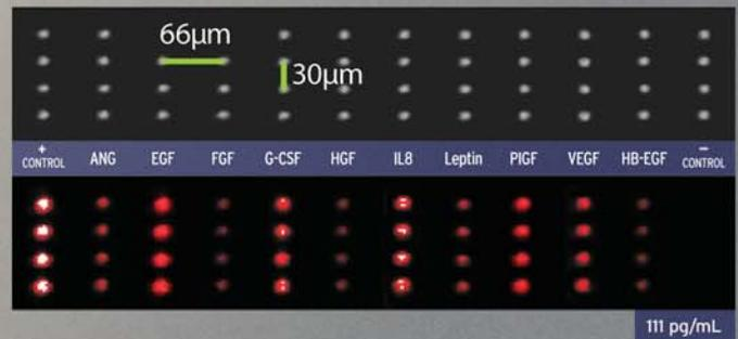
**Top:** Optical image of highly uniform angiogenesis antibody features in one nanoscale sub-array. **Bottom:** Fluorescent image showing ultrasensitive NanoInk assay results using 111 pg/ml of recombinant human antigens.
