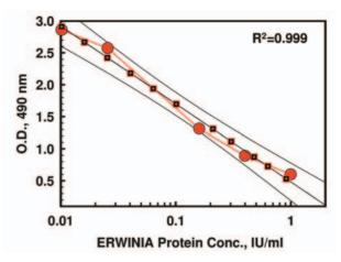
Figure 3. Calibration line showing the relationship between the average Erwinase Protein Vectastain Assay (n=3 in triplicate or n=9)  $\pm$ SDEV  $\pm$ 95% confidence intervals (%CI) diluted in human serum and optical density OD 490 nm response for the Erwinase protein standard solutions.
